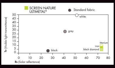
The fabric SCREEN NATURE ULTIMETAL® compared to standard PVC free fabric
